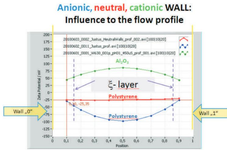
**Fig. 4:** Green: ZP of  $Al_2O_3$  is +50 mV, walls are cationically coated. Red: -25 mV ZP anionic polystyrene, -; the walls are neutral. Blue: polystyrene -40 mV ZP, cell walls are anionic as uncoated glass usually is.
