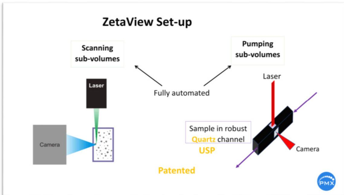
Programming a kinetic measurement where each profile scan is followed by a burst of 5  $\mu$ l new sample, the statistical validity is boosting. See the next slide [\(or Video\)](#):
