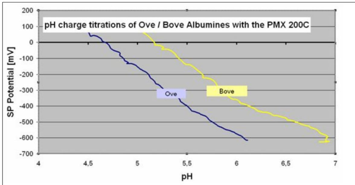
The above diagram shows pH titrations on 10 ml of 1% w/v hen (OVE) and bovine (BOV) albumins. The IEP of the 1 nm OVE albumin is at pH = 4.7, the IEP of the 5 nm bovine albumin is at pH = 5.2. At the end of the titration the samples were coagulated.
