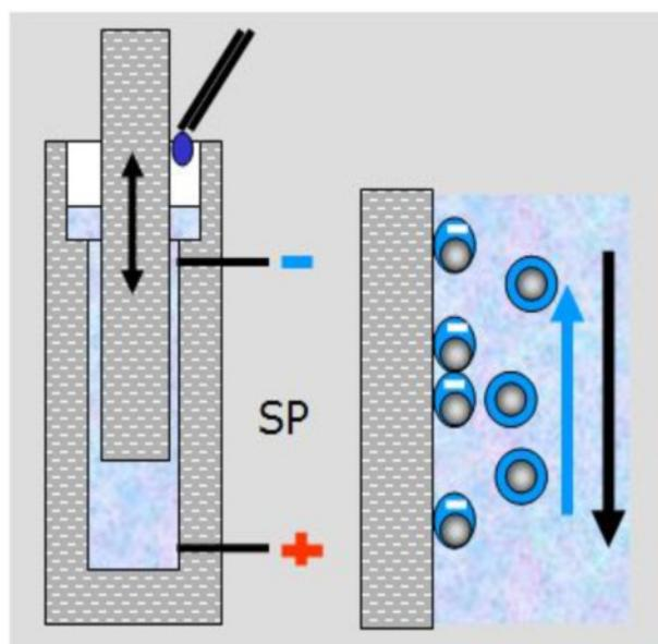
**Stabino® principle:** Piston moving up and down in the measurement cylinder, inducing the particle interface potential **SP** and mixing during auto-titration.
